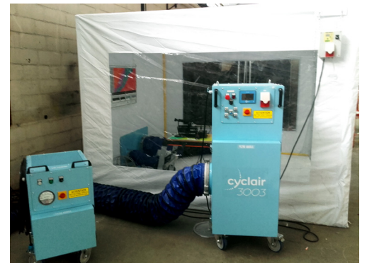
Negative pressure applied to a flexible containment airlock with a CYCLAIR® 3003 and a CYCLAIR® 503
