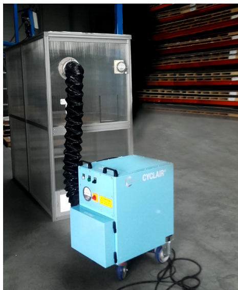
Negative pressure applied to a rigid containment airlock with a CYCLAIR® 502
